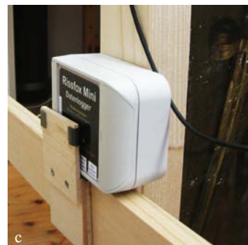
Fig. 51: a. to c. Movement measurements with the potentiometer (Rissfox®).
