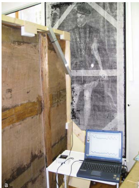
Fig. 51: a. to c. Movement measurements with the potentiometer (Rissfox®).
