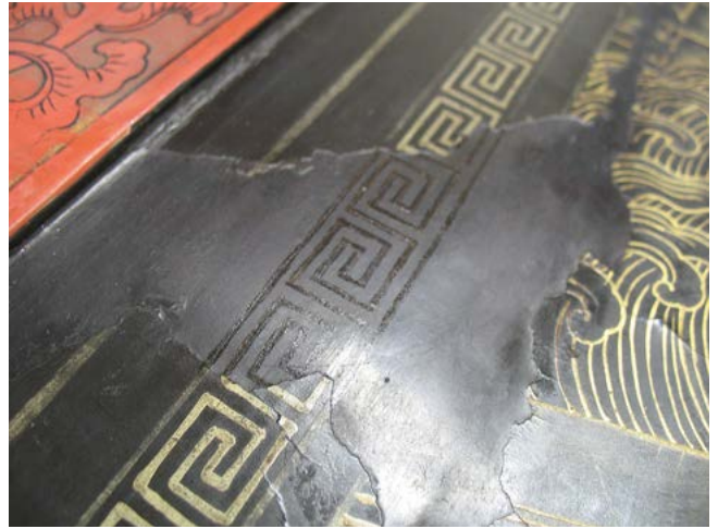
Fig. 87: Reduced (blotted) application of the oil mordant.
