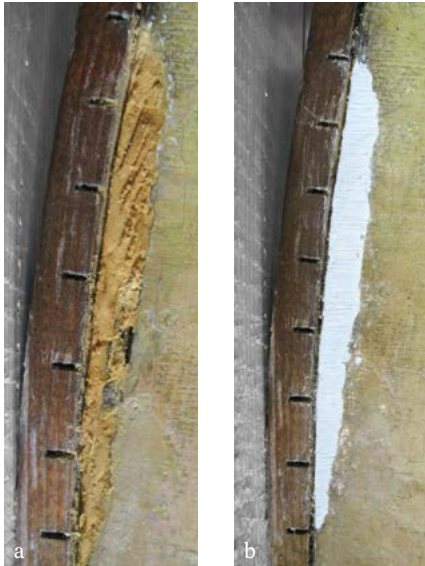
Fig. 56: a. 10 mm wide strip of wood at the edge and filling of woodworm damaged areas with old spruce fibres and wood putty. b. Detail after filling of the loss.
