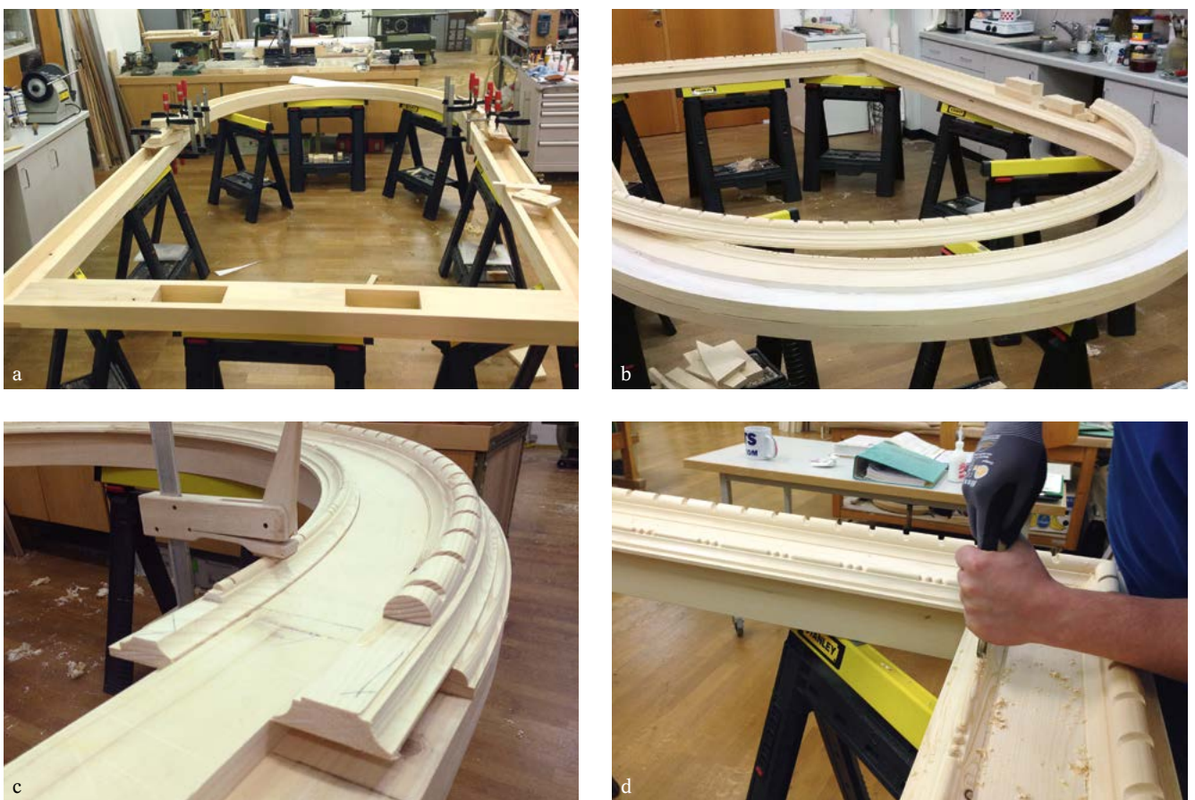
Fig. 61: a. The reverse of the frame during gluing. b. Construction of the face of the frame. c. Joining the individual pieces of wood for the arch. d. Carving ornament with a chisel.
