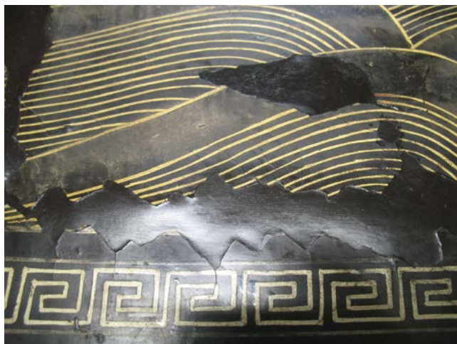
Fig. 85: Compensation in wax with the hardened urushi coating ( suri-urushi ).
